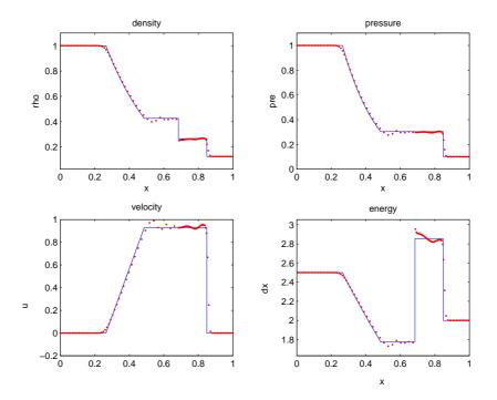
Figure 2.8: Sod's shock tube problem at t=0.2 with bulk artificial viscosity coefficients  $c_l = 0.1$  and  $c_q = 1.0$ .
