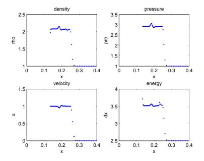
Figure 3.4: Fine-to-coarse 2 region test problem, mesh density ratio 2:1, t=0.13 with  $c_l = 0.1$  and  $c_q = 1.0$ .
