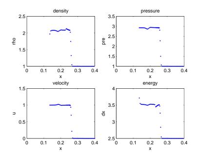
Figure 3.3: Coarse-to-fine 2 region test problem, mesh density ratio 1:2, t=0.13 with  $c_l = 0.1$  and  $c_q = 1.0$ .
