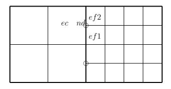
Figure 4.5: Diagram of a course-to-fine interface to show entries of disjoint elementelement array. The empty circle indicates the disjoint node.
