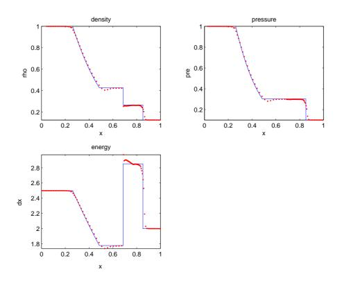
Figure 4.13: Two level adaptive mesh results for Sod problem with Christensen artificial viscosity coefficients  $c_l = 0.5$  and  $c_q = 0.75$  at t=0.2.
