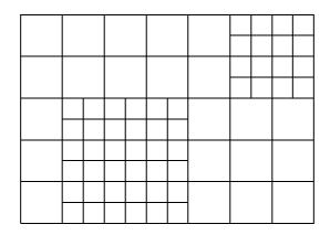
Figure 4.1: Diagram of the dynamic mesh with fine elements inserted.
