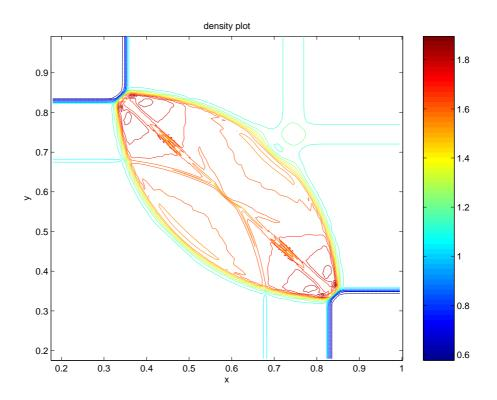
Figure 4.16: Two level adaptive mesh calculation density contours for 2D Riemann problem with Christensen artificial viscosity at t=0.2.
