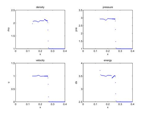
Figure 3.5: Coarse-to-fine 2 region test problem, mesh density ratio 1:3, t=0.13 with  $c_l = 0.1$  and  $c_q = 1.0$ .
