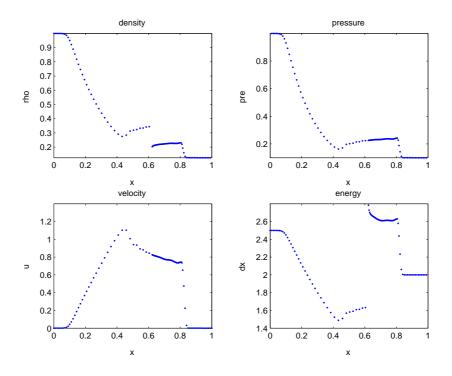
Figure 2.10: Radial Sod problem at t=0.25 with bulk artificial viscosity coefficients  $c_l = 0.1$  and  $c_q = 2.0$ , 200 mesh.
