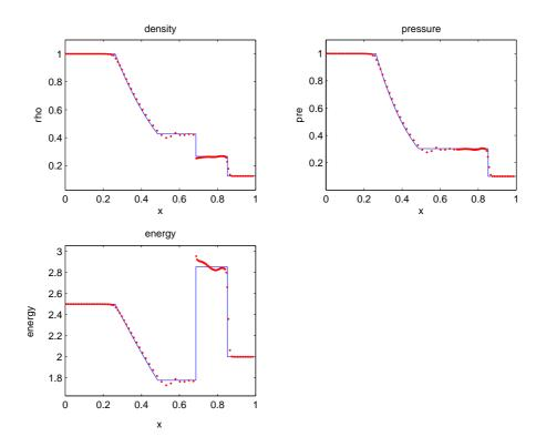
Figure 4.12: Two level adaptive mesh results for Sod problem with bulk artificial viscosity coefficients  $c_l = 0.1$  and  $c_q = 1.0$  at t=0.2.
