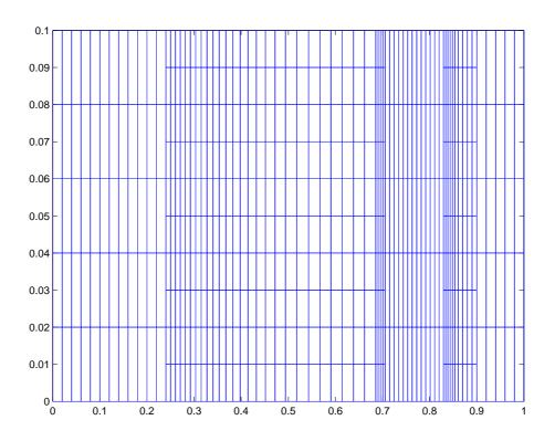
Figure 4.10: Two level adaptive mesh for Sod problem with bulk artificial viscosity coefficients  $c_l = 0.1$  and  $c_q = 1.0$  at t=0.2.
