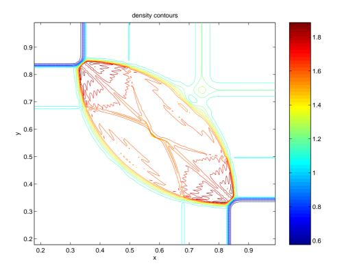
Figure 2.12: Two dimensional Riemann problem 4 shocks, at t=0.2 with bulk artificial viscosity coefficients  $c_l = 0.08$  and  $c_q = 1.0$ .
