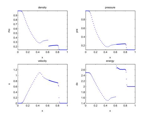
Figure 2.11: Radial Sod problem at t=0.25 with Christensen artificial viscosity coefficients  $c_l = 0.5$  and  $c_q = 0.75$ , 200 mesh.
