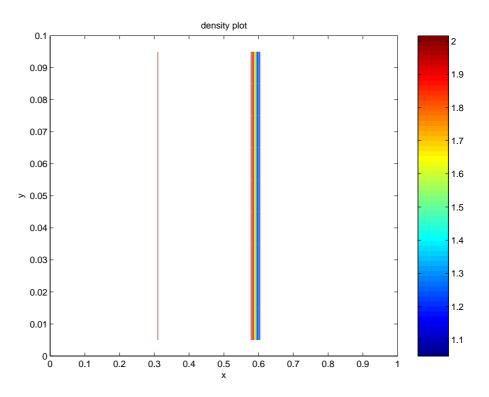
Figure 4.9: Two level adaptive mesh density contours for piston problem with bulk artificial viscosity coefficients  $c_l = 0.1$  and  $c_q = 1.0$  at t=0.3.
