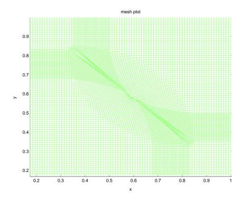
Figure 2.13: Two dimensional Riemann problem mesh 4 shocks, at t=0.2 with Christensen artificial viscosity coefficients  $c_l = 0.3$  and  $c_q = 0.65$ .
