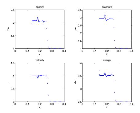
Figure 3.6: Fine-to-coarse 2 region test problem, mesh density ratio 3:1, t=0.13 with  $c_l = 0.1$  and  $c_q = 1.0$ .
