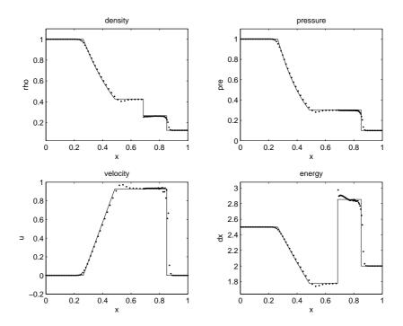
Figure 2.9: Sod's shock tube problem at t=0.2 with Christensen artificial viscosity coefficients  $c_l = 0.5$  and  $c_q = 0.75$ .
