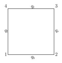
Figure 2.3: Diagram edge viscosities and node numbering. Each node has position (z,r).
