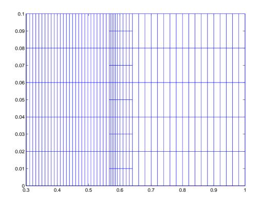
Figure 4.8: Two level adaptive mesh for piston problem with bulk artificial viscosity coefficients  $c_l = 0.1$  and  $c_q = 1.0$  at t=0.3.
