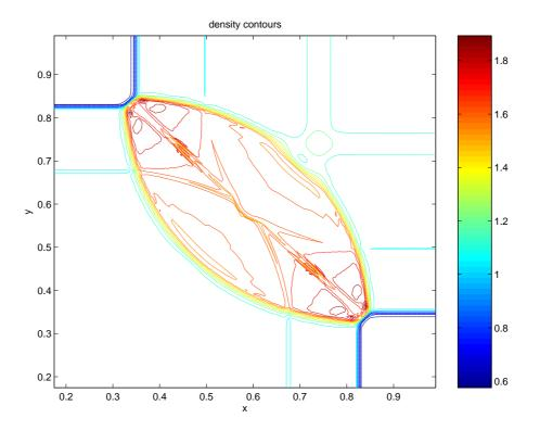
Figure 2.14: Two dimensional Riemann problem density contours 4 shocks, at t=0.2 with Christensen artificial viscosity coefficients  $c_l = 0.3$  and  $c_q = 0.65$ .
