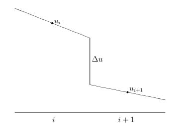
Figure 2.2: Diagram showing the  $\Delta u$  used in Christensen's artificial viscosity.
