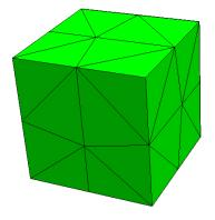
Fig. 6. Unstructured mesh
