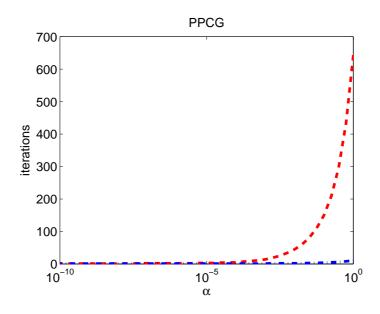
Figure 3: Number of PPCG iterations when either (a)  $\mathcal{P}$  or (b)  $\mathcal{P}_{C}$  are used as preconditioners for  $C = \alpha I$  on the AUG2DQP problem.
