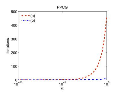
Figure 4: Number of PPCG iterations when either (a)  $\mathcal{P}$  or (b)  $\mathcal{P}_{C}$  are used as preconditioners for  $C = \alpha \times diag(0, \ldots, 0, 1, \ldots, 1)$ , where  $rankC = \lfloor m/2 \rfloor$ , on the AUG2DQP problem.
