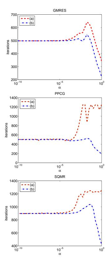
Figure 2: Comparison of number of iterations required when either (a)  $\mathcal{P}$  or (b)  $\mathcal{P}_{_{C}}$  are used as preconditioners for  $C = \alpha I$  with GMRES, PPCG and SQMR on the CVXQP2\_M problem.
