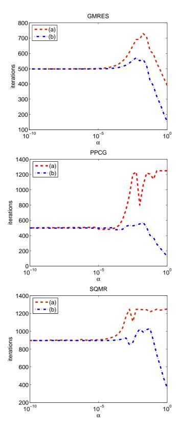
Figure 1: Comparison of number of iterations required when either (a)  $\mathcal{P}$  or (b)  $\mathcal{P}_{_{C}}$  are used as preconditioners for  $C = \alpha I$  with GMRES, PPCG and SQMR on the CVXQP2\_M problem.
