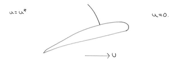
For a steady shock,  $\psi=\psi(\chi)$  , where  $\chi=x$  - Ut is the modified x co-ordinate and  $\psi=u$  , a ,  $\rho$  etc.
