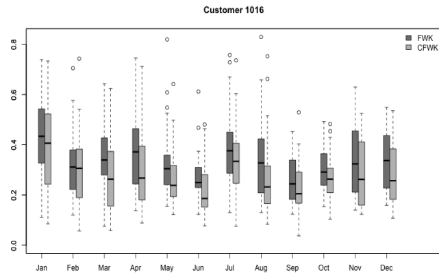
Figure 7: Distribution (by month) of the daily median absolute errors (DMAE) obtained by CFWK and FWK (case of customer 1016).
