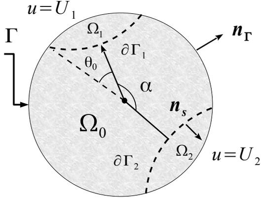
FIG. 2. Illustration of the flow and solution domains on the surface  $\Gamma$  of a spherical particle, and their geometric arrangements. In the picture,  $\Omega_0$  is the domain of the surface flow and the surface area covered by the liquid bridges corresponds to the domains  $\Omega_1$  and  $\Omega_2$ .
