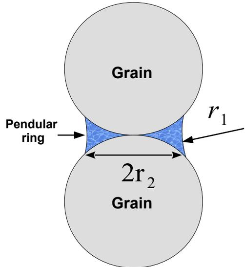
FIG. 5. Illustration of the pendular ring characteristic geometry.
