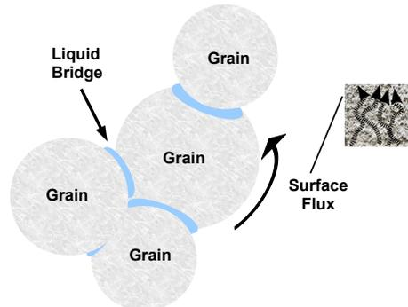
FIG. 1. Illustration of the liquid distribution in particulate porous media (grey) with pendular rings (blue) at low saturation levels.
