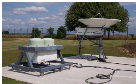
Figure 3.17: Image of the Galileo (left) and Copernicus (right) radars at Chilbolton observatory in Hampshire. The data in this study is taken from Copernicus, the 8.6mm radar. This image is taken from [37]
